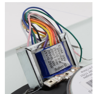
70/25V transformer with colored leads
