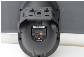
Transformer Dial & Terminals
