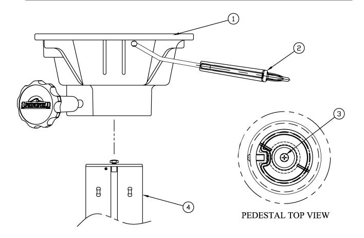
After placing your Springfield <u>Marine</u> Slide or Swivel (Item #1) onto the pedestal (Item #4) verify that the pedestal adjustment handle (Item #2) is functioning properly.
