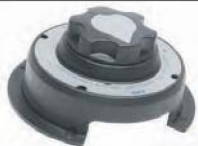
UM-44 BATTERY SELECTOR & DISCONNECT SW. 4 position {OFF - ON - Battery No.1 ON - Both Batteries - ON Battery No. 2.} Flange dia. 6" height 2 5/8". Rating: 310 Amps. cont, 500 Amps inter, 6 - 36 Volts, D.C
