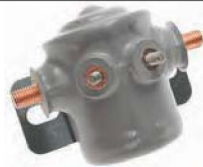
UM-48 SOLENOID - H.D. Circuit 4,12 Volt. Weather resistant, continuous & intermittent type. Intermittent rating: 750 Amp. make - 100 Amp. break 10 sec. ON, 30 min. OFF. Continuous rating: 85 Amp.-12 Volt DC
