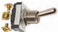
DS-128 TOGGLE SWITCH - Single pole, double throw, {ON- OFF-ON}. Underwriters approved. Mounting stem dia. 15/32", length 1/2". Rating: 125 Volts 15 Amp. - 250 Volts 10 Amp. 3/4 H.P. 120-240 Volts AC.
