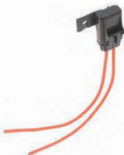
FH-25 FUSE HOLDER - Single sealed with latching Nylon cap, silicone rubber seals. Leads 9", 12 gauge wire. Will fit blue butt conn. for splicing into 14, 16 and 18 gauge applications. Rate
