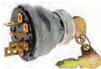
UM-124KA IGNITION SWITCH - 3 position w/ anti-restart. Keyed alike. Must be turned {OFF} before it start again, key removable in {OFF} position. Mounting stem dia. 1", len., 23/64" 12 Volt D.C. 10 Amp. 12 Volt
