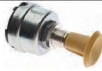
DS-133 PUSH-PULL SWITCH - w/ plastic knob, ceramic base, & 2 screw term. Mounting stem dia. 15/32", length 1/2". Rating: 6 Volts 35 Amp. - 12 Volts, 20 Amp.
