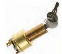
US-129 IGNITION SWITCH - Brass, 4 positions - ACC {OFF} - IGN & ACC {Start}. Spring loaded. Mounting stem is 13/16" dia, 1-7/32" long. Keyed removable in {OFF} position only.
