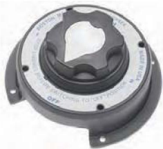
UM-47 BATTERY SELECTOR & DISCONNECT SW. 6-36 Volts, D.C. 4 position, {OFF - ON-Battery No.1 -ON-Both Batteries - ON-battery No. 2.} Rating: 310 Amps. Continuous, 500 Amps. Intermittent.
