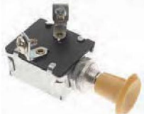
DS-123 PUSH-PULL SWITCH - Single pole, single throw. Pull-{ON}, Push-{OFF} switch. With large plastic knob, and 2 screw terminals. Mounting stem dia. 15/32", length 1/2". Rating: 6 Volts 20 Amp. - 12 Volts
