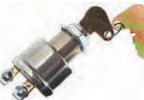
UM-125KA MAGNETO IGNITION SWITCH - Lock cyl. & keys, keyed alike. Switch has 3 positions, weatherproof O-Ring seals, and 3 screw term. Mounting stem dia. 5/8", length 3/8".
