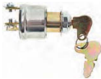
UM-123KA IGNITION SWITCH - w/ lock cyl & keys, keyed alike. 3 positions, weatherproof O-Ring seals. Key removable in {OFF} position only. Mounting stem dia. 5/8", len 7/16". 12 Volt D.C., 5 Amp.
