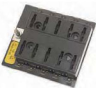
FH-26 FUSE BLOCK - For ATC or ATO fuses or Plug in Circuit Breakers. Max. per circuit at 12V (DC), 150 Amp. total for block at 12V (DC), for 24V (DC) use only ATC or ATO fuses. Total of 10 Fuse or Breaker.
