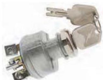
UM-41 IGNITION SWITCH - Similar to {US-126KA} except with screw terminals. A special ratchet prevents the key from being turned to the {Start} position without first going all the way to the {OFF} position
