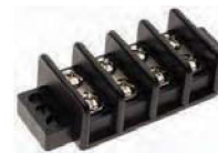
JB-5 JUNCTION BLOCK - 300 Volts, 30 Amps. 4 gang, with brass plated links and terminal screws. Has two 7/32" diameter mounting holes on 2-3/4" center.
