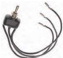
UM-45 TOGGLE SWITCH - {OFF-ON}, S.P.D.T. 16 ga leads. Mounting stem 15/32"-32, 13/32" long. Fits panels up to 3/16" thick. Rating: 25 Amps. -Lamp load 35 Amps. -Inductive Load.
