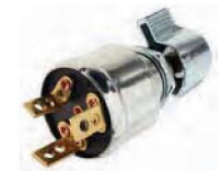
US-128 IGNITION SWITCH - 3 postions {OFF}-{IGN}-{START}. Spring loaded. Mounting stem is 5/8" dia, 7/16" long. Weatherproof ring seals. Rating: 12 Volt D.C., 10 Amp. ignition. 12 Volt D.C., 5 Amp. start.
