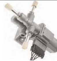
FV-6 FUEL SELECTOR - 3 Port Motorized Valve and Connector. Meets USCG regulations. Used w/ twin permanently installed gasoline fuel tanks, 12 VDC electrical system & 3/8" I.D. hose.
