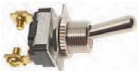
DS-116 TOGGLE SWITCH - 2 position, single pole, single throw. UL approved. Mounting stem dia. 15/32" length 3/8". Rating: 125 Volts 10 Amp. - 250 Volts 5 Amp.
