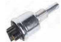
US-127 IGNITION SWITCH - with Lock Cylinder. Two position. {OFF}-{ON}, with 2 screw terminals. Mounting stem 1/2" diameter, 1/2" long. Rating: 10 Amp. at 12 Volt D.C.
