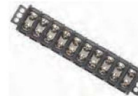
JB-4 JUNCTION BLOCK - 10 gang, w/ brass nickel plated links and term screws. Has 7/32" dia mounting holes on 6-3/16" center.
