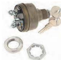
US-72 MAGNETO IGNITION SWITCH - w/lock cylinder & keys. 4 position, 5 screw term, magneto grounded in "OFF" position. 3/4"-20 Thread.
