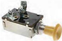
DS-120 PUSH-PULL SWITCH - Heavy duty, 2 position, single pole, single throw, Push-Pull switch. With knob and 3 screw terminals. Mounting stem dia. 7/16", length 1/2". Rating: 6 Volts 30 Amp. - 12 Volts 15 A
