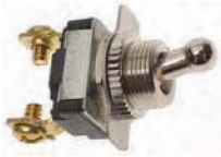
DS-122 TOGGLE SWITCH - 2 position, single pole, single throw. Underwriters approved. With 2 screw terminals. Mounting stem dia. 1/2" length 1/2". Rating: 125 Volts 6 Amp. - 250 Volts 3 Amp.
