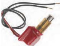
UM-46 PUSH BUTTON - 2 positions, OFF-MOMENTARY ON. w/ button depressed, spring return to OFF. 18 ga. copper leads. Mounting stem 5/8"-32, 25/16" long. Fits panels up through 1/2" thick.
