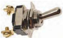
DS-126 TOGGLE SWITCH - Heavy duty, 2 position, single pole, single throw With {OFF-ON} face plate and 2 screw terminals. Mounting stem dia. 15/32", length 3/8". Rating: 6 Volts 35 Amp.
