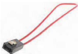
FH-20 FUSE HOLDER - Single heavy dut supplied with 18" loop of 12 gauge UL-1015 wire that can be cut to length. Wire meets recreational vehicle industry specifications. Rated 3-30 Amps.
