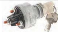
US-126KA IGNITION SWITCH - w/ anti-restart, pick-proof lock, keyed a like. 4 positions, O-Ring seal. Mounting stem dia. 3/4", length 7/16" 12 Volts, 8 Amp Ignition. 12 Volts, 30 Amp. start.
