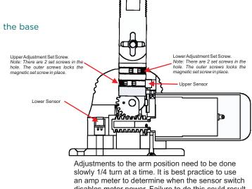
disables motor power. Failure to do this could result in motor failure.
