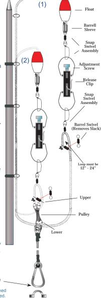
When trolling with outriggers you can troll with more lines in the water, thus pulling more bait which simulates a school of fish. Outriggers will eliminate tangled lines. Each outrigger can accommodate one or two lines from your rods and reels. The line is used with a release clip that extends to the end of your outrigger. When a fish strikes your bait, the release clip will allow your fishing line to come free of the outrigger so you can reel in the fish.
