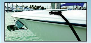
Taco Marine's convenient Rub Rail Kits include rub rail (in a continuous coil for one piece installation without seam), insert, end caps (where applicable) and screws.
