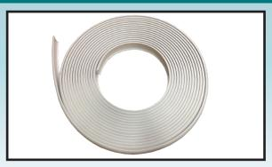
Taco Marine's latest Rub Rail innovation is an improved design of our most popular rigid PVC shape with a light weight, high-density inner core. This allows for easier handling, faster one-piece installation, improved dimensional stability and production run consistency. It receives the S11-4511 ¾" hollow back Stainless Steel half-oval insert and is ideal for boats up to 40' in length.
