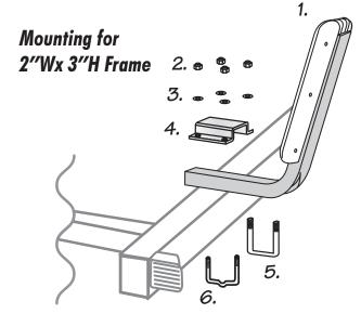
NOTE: On 2"W x3"H tube the u-bolts are not "Cross mountined".
