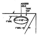
4. Using your location marks, drill out the holes for the new fill, (2" dia. with the edge of the hole 1" minimum from the edge of the tank), supply and/or vent
