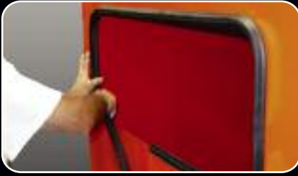
1. Secure Locking Gasket to body panel.
