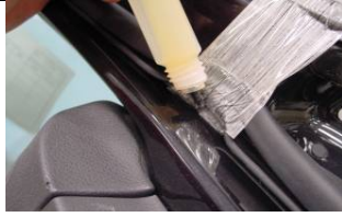
Terokal® adhesive applied to gapped section of seal.
