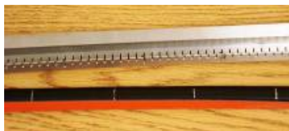
Seal marked every 10 cm with silver marker; shown with the marking fixture.
