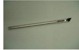
Artist's brush may allow better control of the amount of adhesive used.
