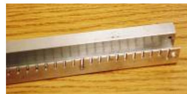
Close-up view of seal marking fixture. Deeper slits are made each 10cm, smaller slits are 1cm apart.
