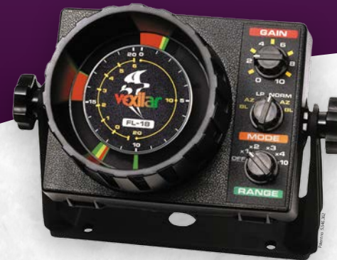
FL-18® Flasher FM1887 with 12° Puck Transducer FM1884 with 12° High Speed Transducer
