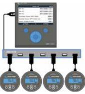
A maximum of four BMVs can be connected directly to a Color Control GX.
