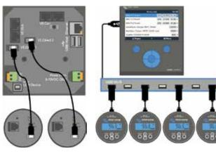
A maximum of four BMVs can be connected directly to a Color Control GX. Even more BMVs can be connected to a USB Hub for central monitoring.
