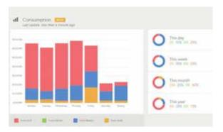
When the Inverter RS is connected to a GX device with internet connection, you can access our free remote monitoring website (VRM). This will display all your system data in a comprehensive graphical format. System settings can be changed remotely via the portal. Alarms can be received by email.
