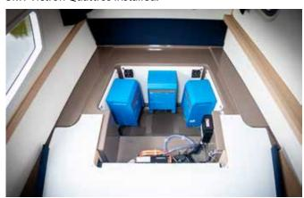
These Quattros convert the 12-volt battery voltage to the 230 volts needed for all 'domestic' electrical appliances. Thanks to the Quattros' high charging capacity, the batteries can be charged quickly, which reduces the number of generator running hours. All power is stored in six Victron lithium batteries with a total capacity of 900 Ah and the 12-volt system installed by the shipyard can continue to be used.
