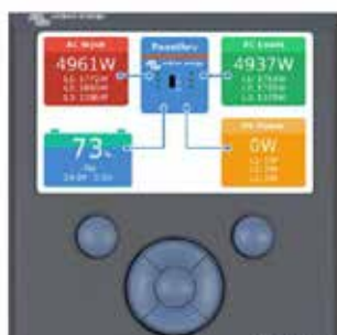
Color Control GX, showing a PV application
