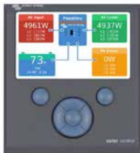
Color Control GX, showing a PV application
