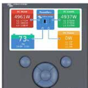
Color Control GX, showing a PV application
