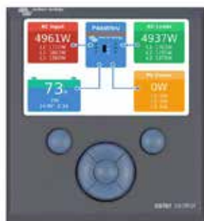
Color Control GX, showing a PV application
