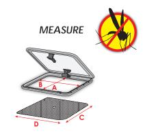
A x B max. 300 x 300 mm (12" x 12") C x D 350 x 350 mm (14" x 14")
