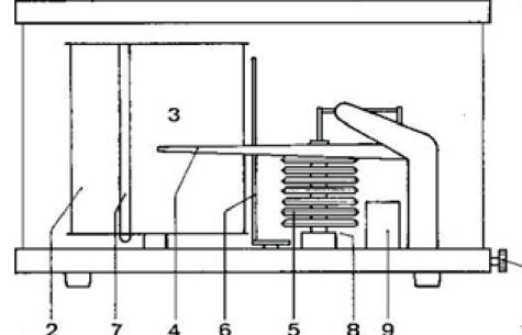
Precision Barograph 4 Diaphragms Quartz movement for chart drum Power supply: 1 x 1.5V AA (incl.) 52- one week charts in inches (incl.) Chart size: H 2" (5.5cm) x L 9 ¼" (23.5cm) Resolution: 2hPa Operating Range: 960...1050hPa Linearity deviation: +-1hPa between 980...1030hPa Case: Mahogany & glass Case dimension:  $7^{3}$ 4" x 5" x 5¼" (197 x 127 x 133mm) Weight: 3 lbs (1.36kg)
