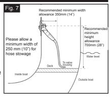
**Please note:** Before installing, ensure that sufficient space is allowed for the shower hose when stowed. Also ensure that it is free from obstructions when pulled out.
