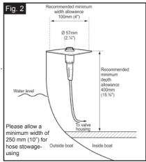
**STEP 2.** Allowing for the height and width restrictions indicated in Fig. 2, drill one 50mm (2") diameter circular hole in the bulkhead above the water line. (See Fig. 3) Please note: minimum mounting surface thickness: 3mm (1/8"); maximum mounting surface thickness 19mm (3/4").
