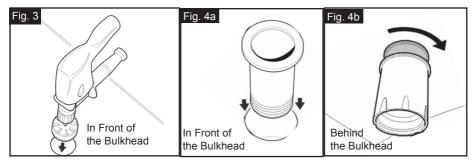
**STEP 3** Place the housing through the hole. Secure by hand tightening the lock nut onto the housing behind the bulkhead. (See Fig. 4a and 4b)
