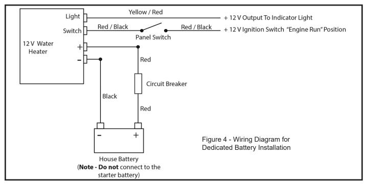
**NOTE:** On 12 volt circuits a 35 amp circuit breaker **must be** used.
