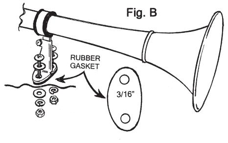
**IMPORTANT:** Make sure the hole is free of any burrs that could cut into the horn's wire. For roof mount mounting, to prevent water leaks, it is recommended that silicon or a waterproof sealer be placed on the wire at the point of entry into the roof.
