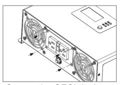
Secure the GFCI device to the inverter unit with the four screws from step 3.
