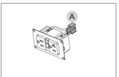
Take the GFCI device out of its box. It comes with an attached connector A.
