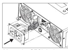
Mount the GFCI device onto the inverter unit.
