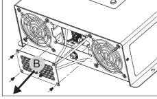
Remove the four screws and detach the GFCI cover plate B from the inverter unit.
