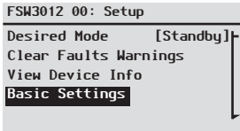
Figure 21 Selecting Basic Settings From the Device Setup Screen
