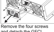
Remove the four screws and detach the GFCI cover plate B from the inverter unit.
