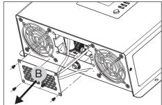
Remove the four screws and detach the GFCI cover plate B from the inverter unit. Set aside the screws.
