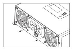
Secure the GFCI device to the inverter unit with the four screws from step 3.
