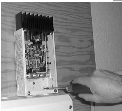
Figure 2-3 Mounting the C-Series Multifunction DC Controller
