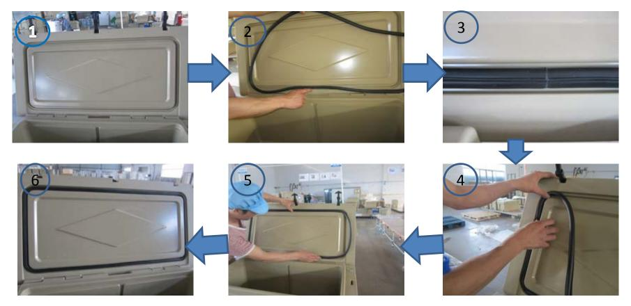
Assemble the gasket to the cover groove
